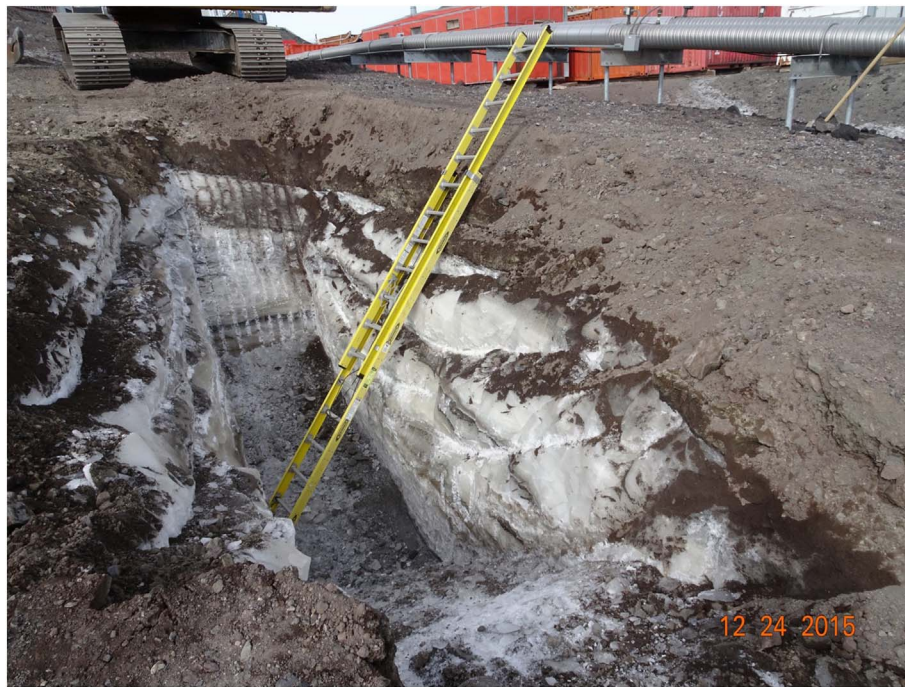
Fig. 11. Photo of the pit 4 showing massive ice buried beneath a shallow cover of stratified thawed and frozen fill.
